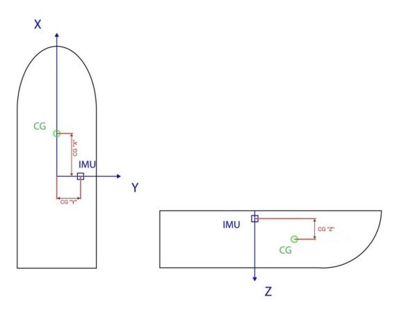
**Lever Arm X** is the fore aft distance in meters between the Motion Sensor and the Lever Arm position. Where a positive distance represents that the Lever Arm measurement point is located fore of the Motion Sensor physical location.
