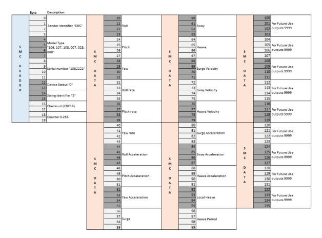
The UDP 2 protocol uses the IEEE Standard 754 representation of the float numbers. In the output message fields, no scaling for the motion sensor data is used when converting from Hex representation to the float values.
