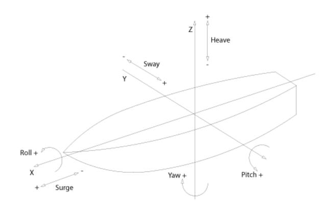
In the SMC motion sensors, the coordinate system can be defined by a setting option in the SMC Configuration software that is included with the motion sensor. The user can choose between the IMU Coordinate system and the Earth Coordinate system. The IMU Coordinate system is the vessel coordinate system when the motion sensor is aligned with the vessel mechanically and/or by offset entries to the motion sensor.
