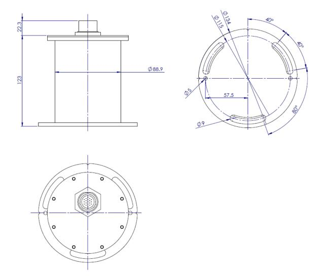
**Note** the IMU base plate has two 5mm holes for mounting and alignment. SMC recommend using 4mm spring pins. The spring pins are an interference fit in the optional mounting bracket plate but should be a push fit in the IMU base.
