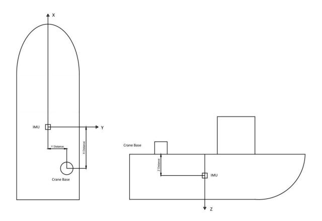
"Remote heave X" is the fore aft distance in meters between the IMU and the crane base. Where a positive distance represents that the motion sensor is located aft of the crane base
