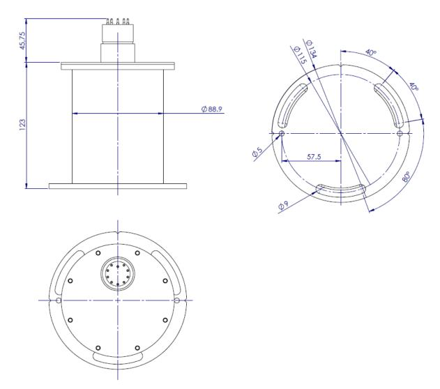
**Note** the IMU base plate has two 5mm holes for mounting and alignment. SMC recommend using 4mm spring pins. The spring pins are an interference fit in the optional mounting bracket plate but should be a push fit in the IMU base.
