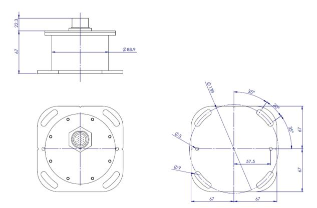
**Note** the IMU base plate has two 5mm holes for mounting and alignment. SMC recommend using 4mm spring pins. The springs pins are an interference fit in the optional mounting bracket plate but should be a push fit in the IMU base.
