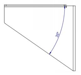
IMU bracket base plate
