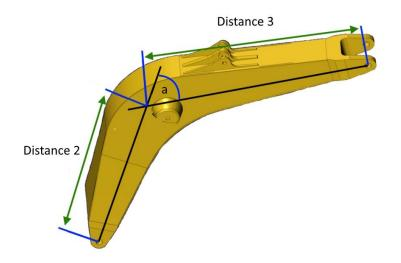
For example, if Distance 2 is 3m and Distance 3 is 3m with an offset angle (**a**) of 35 degrees between them, the crane below will be drawn.
