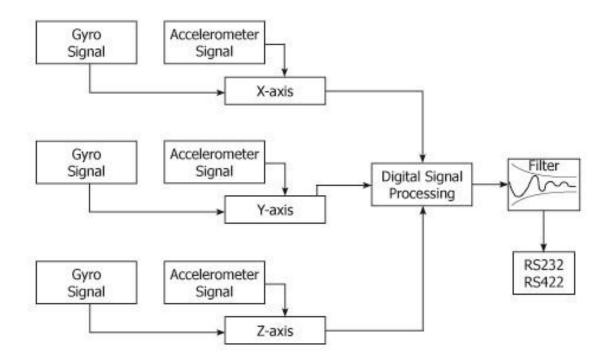
Heave, surge and sway are calculated by integrating the acceleration in the X, Y and Z axis twice. The integrated data is filtered with a high pass filter. The calculations of the distances are optimized for continuous motion and not for static distance measurements, as the high pass filter will filter the position over time to zero. The dynamic motion filtering is designed to measure motions over a period between 1 s and 25 s.
