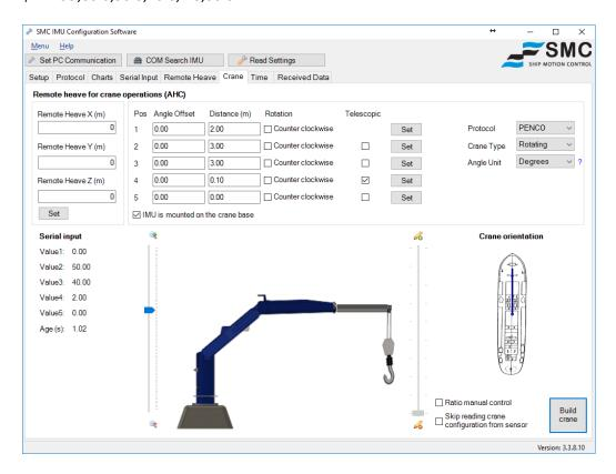
Now the encoder Value 4 is zero and the telescopic arm is fully retracted. \$PENCO,00.0,50.0,40.0,**00.0**,00.0
