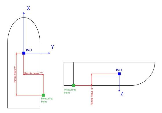
**Remote heave X** is the fore aft distance in meters between the Motion Sensor and the remote heave point. Where a positive distance represents that the remote heave measurement point is located fore of the Motion Sensor physical location.
