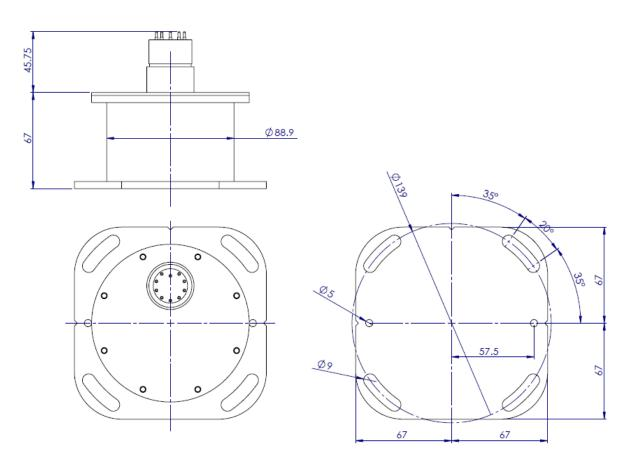
**Note** the IMU base plate has two 5mm holes for mounting and alignment. SMC recommend using 4mm spring pins. The springs pins are an interference fit in the optional mounting bracket plate but should be a push fit in the IMU base.
