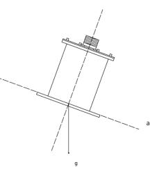
For the Roll, Pitch and Yaw calculations which are always in the Earth Coordinate system, the threedimensional rotation corresponding to the motion sensor readings is composed (conjugated) with the three-dimensional rotation of the mounting offsets. The roll, pitch and yaw velocities being output in the earth coordinate system are the derivatives of the corresponding angular values.
